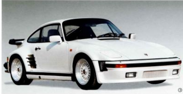
EXC 02 Luftzufuhrhäkchen an hinteren Bodenschwelle EXC 02 Air intake ducts on rear fenders
